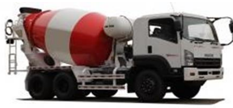
Gambar 7. Concrete Mixer truck Sumber: Tractors, (2019)
